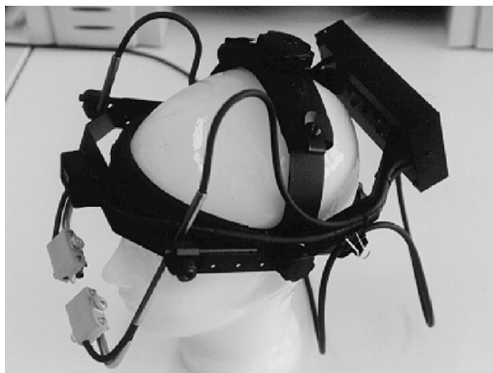
Figure 6: The eye tracker headset of the SMI EyeLink System (Pomplun (1998))
