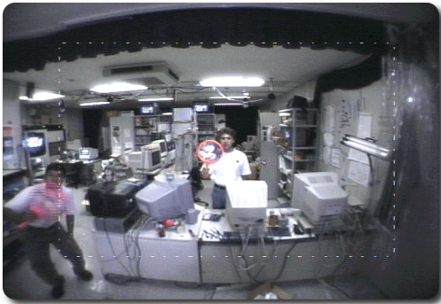
Figure 2.6: Focused object (sign with red boundary) after head-eye saccade, taken from [VCSS01].
