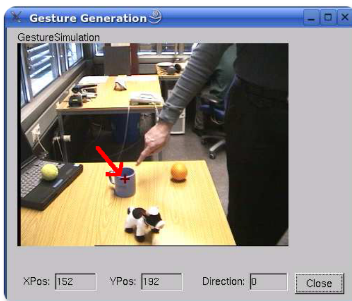
Figure 3.7: Touch screen functionality of the Object Attention System. Image adapted from [Sae05].
