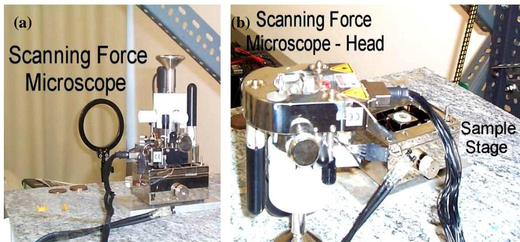
**Figure 4.14** (a) and (b) Photos of Topometrix AFM microscope as used in this work for topography and magnetoresistance map measurement.
