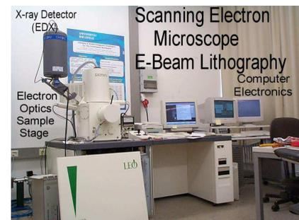
**Figure 4.7** Photograph of the scanning electron microscope Leo 1530.
