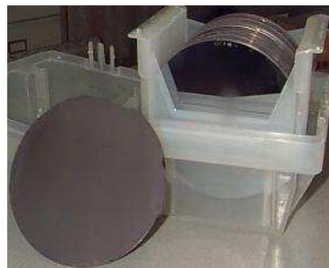
**Figure 4.1** Silicon wafers.
