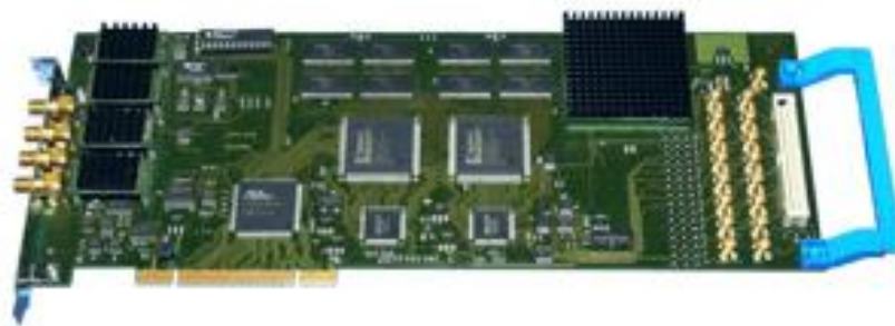
Figure 3.2: The DPC-230 module. It is a single slot PCI module with operating software for Windows 2000, NT and XP. It has 16 LVTTL inputs and 4 CFD inputs and is able to record absolute photon times with time tags.
