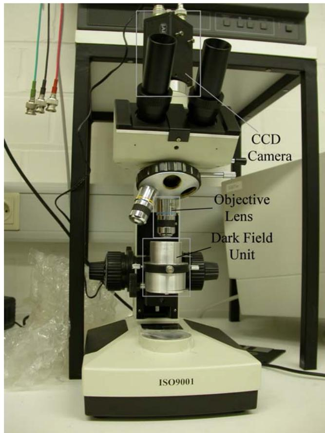
Fig. 2-13: Set-up for the validation of the manufactured dark field illumination unit on a normal microscope.
