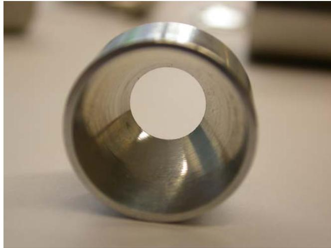
Fig. 2-11: The dark field condenser lens that has been designed and manufactured.
