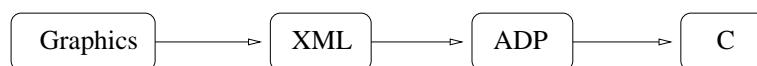
Figure 5.1: The graphical programming system is composed of 4 layers from graphics via XML and ADP code to an executable C-program.
