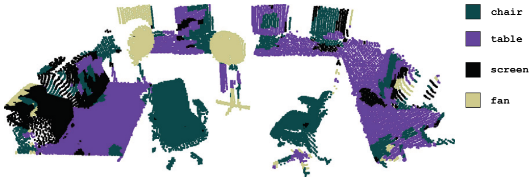
Figure 4.3: This figure shows a semantic labeling of 3D points of an indoor scene using the point-based classification proposed by Triebel [Trio7].
