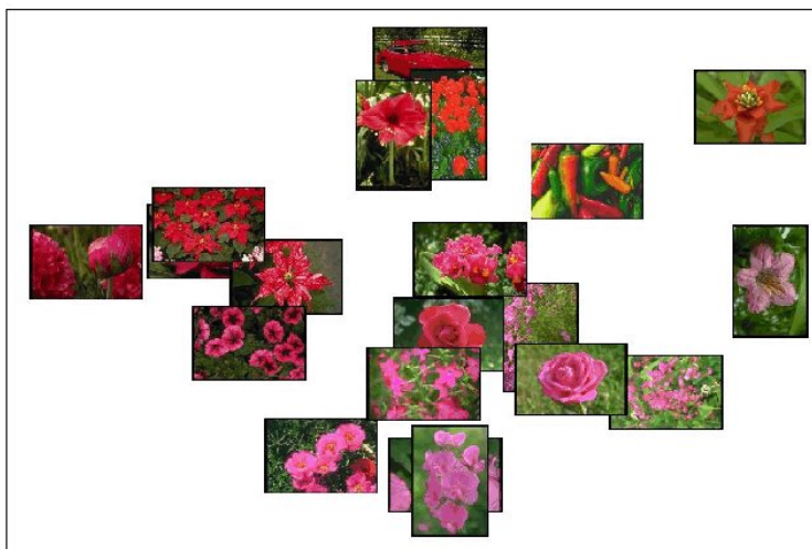
Figure 5.1: MDS display of a query result where the user was looking for flower images from an image set of 20000 images (from Rubner & Tomasi, 2001, p. 83). The images are arranged from pink to red flowers on one axis and according to the shades of green on the other axis.
