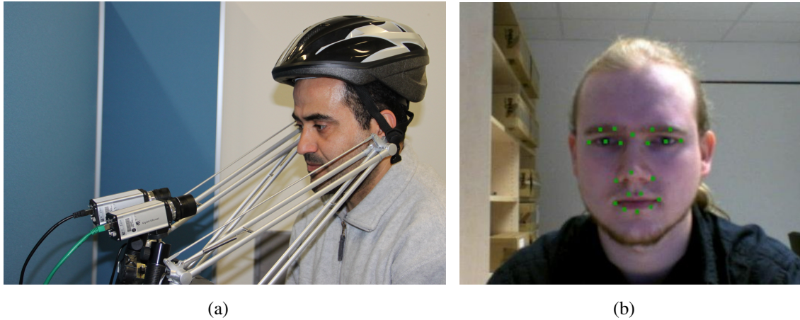
Figure 4.2: Special constrained conditions of facial expression analysis systems. (a) Two cameras are mounted to an arrangement that keeps the head fixed in order to enable the system to capture specific views of the face. (b) The face is labeled with colored markers; they are tracked to infer some emotion-related displacements.
