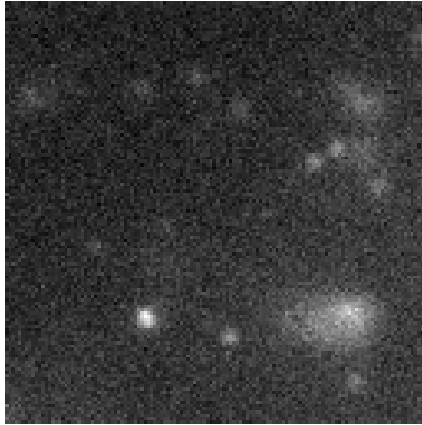
Figure 4.1: Typical dSTORM source image. This is image 34 of the stack that will be labeled as specimen 1. The fluorescent spots show different intensities and forms; note the blurry residual in the upper right corner, probably some out-of-focus fluorophore, and the strange structure in the lower right corner. The distance between pixels in the object plane was estimated to 71 nm.
