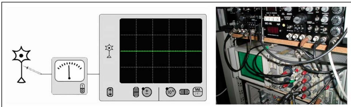
**fig. 2: Experimental setups.** On the left side, a schematic representation of a simple experimental situation is shown. From left to right a neuron's electric activity is registered with a microelectrode, processed through metrology and visualized on an oscilloscope. © 2000 rubin, (permitted reprint). The photograph of metrology used in brain studies on the right side illustrates that laboratory setups are usually much more complicated than suggested in the scheme.
