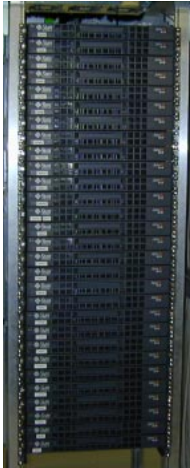
Figure 4.18.: The compute cluster of the Center for Genome Research at Bielefeld University. 30 Sun Netra t1(105) workstations with Ultra Sparc IIe CPUs (360Mhz, 128 MB RAM)
