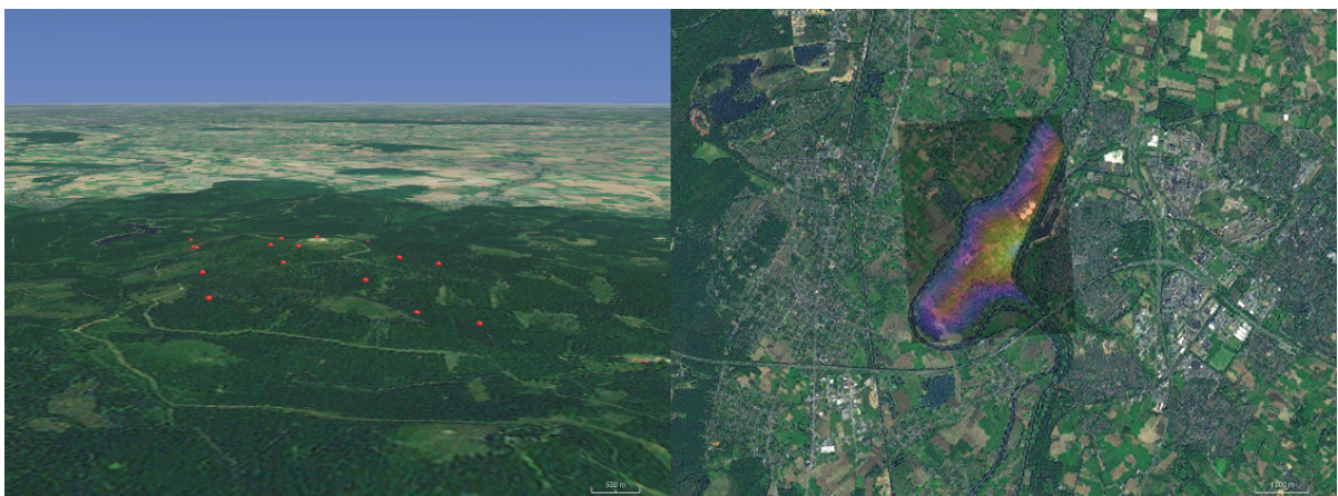
Figure 33: Left: Dynamic data visualized as spheres on the WorldWind globe; Right: Georeferenced data (Meuse data) from "R" and plotted with accurate coordinates on the globe. The meuse data set used here as an example is a data set comprising of four heavy metals measured in the top soil in a food plain along the river Meuse (Netherlands; Lat: 50.9703 Lon: 5.7415 – WGS 84).
