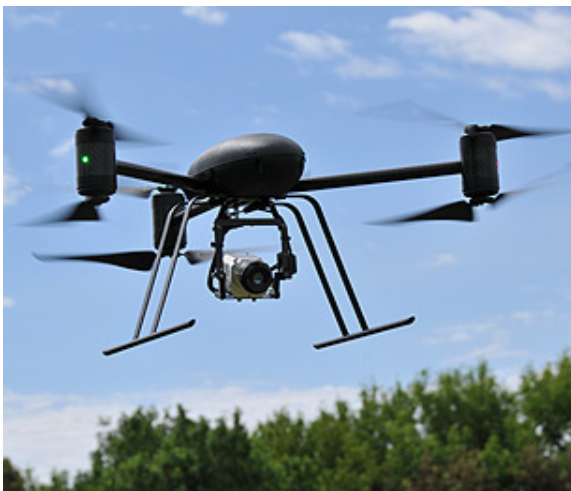
Figure 50: UAV equipped with a digital camera (image from Draganfly Innovations Inc. www.draganfly.com )
