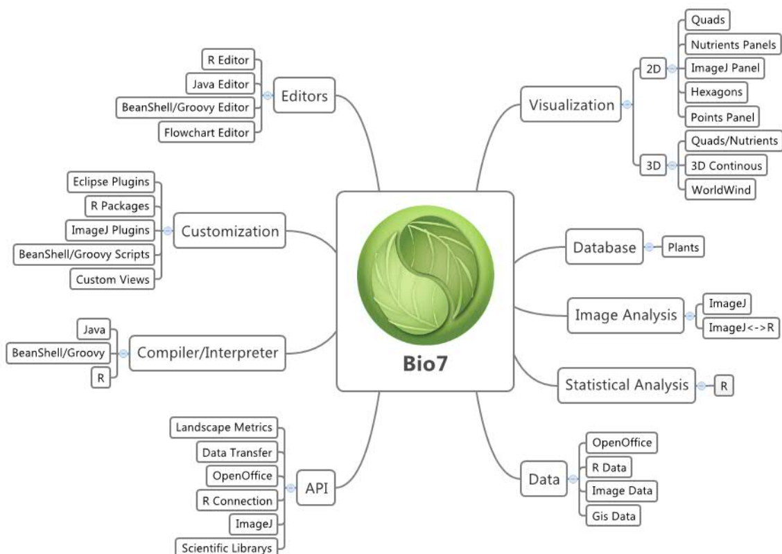
Figure 25: Components of the Bio7 application
