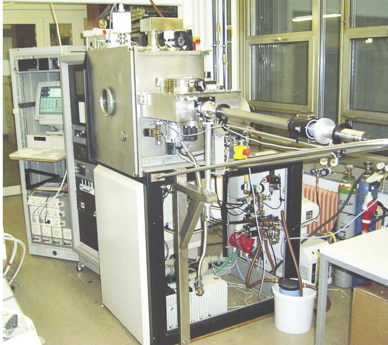
Figure 3.4: Sputter device lab 560 from Leybold.
