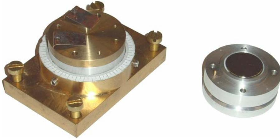
**Figure 4.22:** Picture of new sample stage with piece "c" between piece "a" and on top piece "d". Besides is visible piece "b" with the permanent magnets inside.
