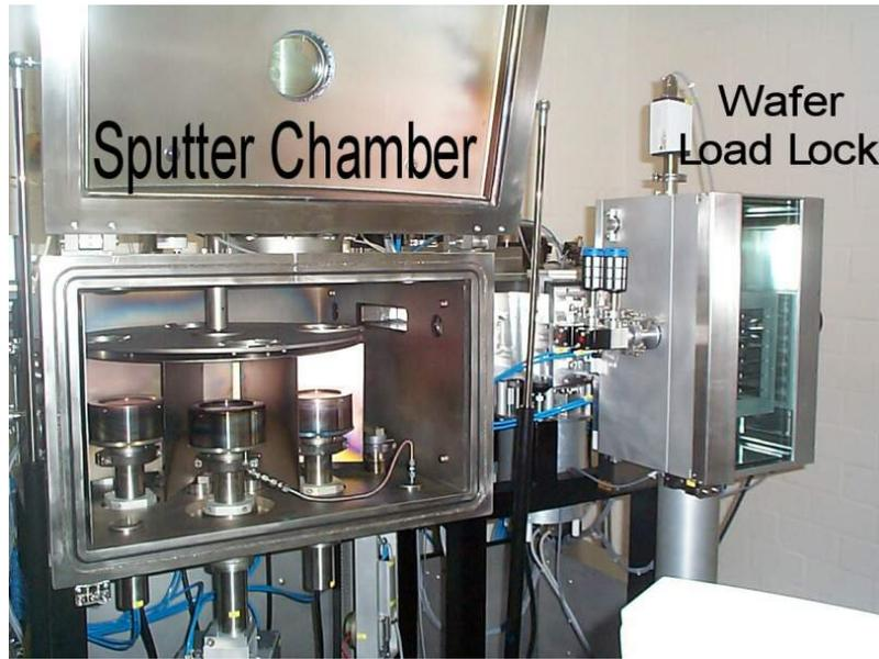
**Figure 2.1:** CLAB 600 – main chamber and load lock. (Taken from "D2 – lab tour" at [www.spinelectronics.de](http://www.spinelectronics.de).)
