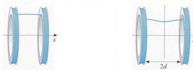
**Figure 1.4:** Sketch of Helmholtz-coils. The line between the coils indicate that for a distance which is equal to the radius, see the left part, one gets the strongest and most homogenous field (after [Mes04, p. 452]).
