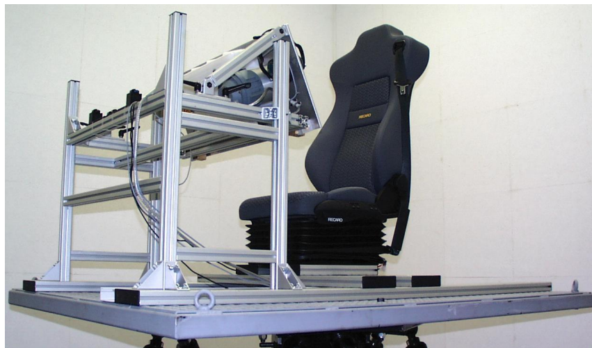
Figure 2.20: Driving setup with force feedback steering wheel.
