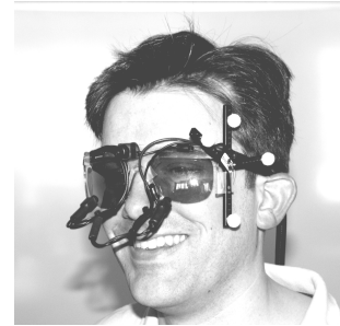
(b) Eye tracker mounted with markers for optical tracking
