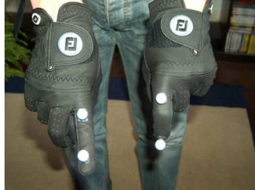
(b) Self-made soft gloves for optical tracking of the index finger
