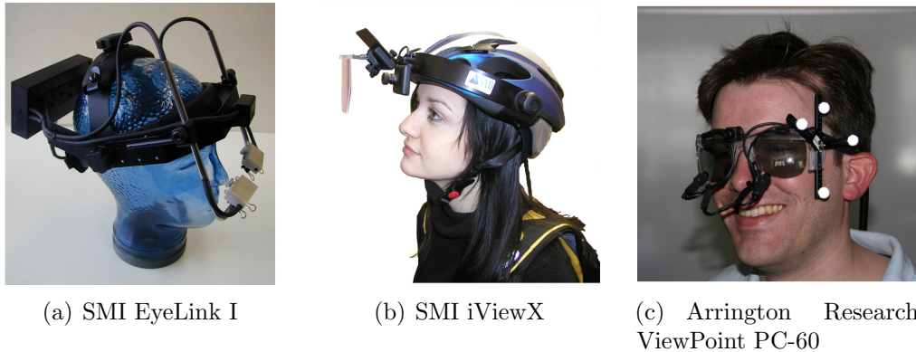
Figure 3.5: A broad range of eye-tracking devices is available. The pictures show different head-mounted devices that may be used in Virtual Reality. The trend in development goes towards more lightweight devices, such as the SMI iViewX or the Arrington Research ViewPoint PC-60.
