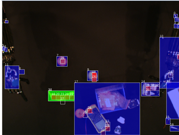
Figure 8.3.: Output of the region selection visualization – best viewed in color. The rectangles shaded in blue are candidates for object detection, the red rectangles are salient points and the green rectangle is the region selected for interaction. Please note that this screen-shot was taken during maintenance of the robot.
