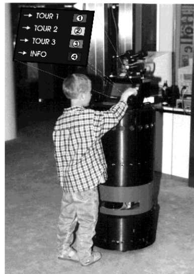
Figure 2.1.: User interface of Rhino, the mobile tour guide robot (from Burgard et al., 2000).
