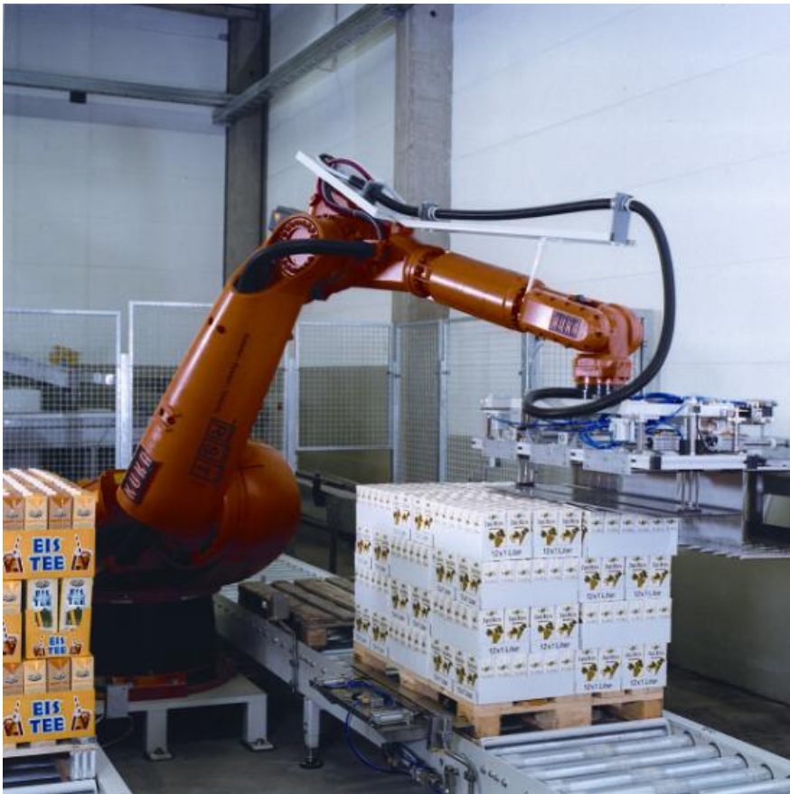
Figure 1.1: KUKA industrial robot - An example of an industrial robot handling drink cartons. Image source: KUKA Roboter GmbH. Reprinted with permission.
