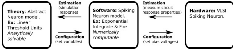
Figure 1: Overview of the parameter translation method for configuring VLSI neurons: How abstract, software, and hardware models of neurons are related and can be used for parameter configuration. The left box represents the set of abstract models that can be analytically solved. The middle box represents the set of spiking neuron models that are typically simulated in software. The right box represents the set of VLSI implementations of spiking neuron models. The left-pointing arrows indicate how parameter estimation is achieved by using observations and measurements from hardware and software models. The right-pointing arrows indicate the parameter configuration process, which originates with the desired biologically relevant variables, and ends with chip biases.
