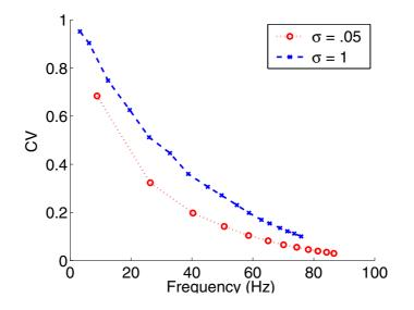
Fig. 5. Coefficients of variation of the I&F neuron's ISIs for two different values of  $\sigma$  plotted against output frequency. Higher  $\sigma$ 's produce higher spike decorrelation, similar to what is observed in Poisson processes (CV close to one).
