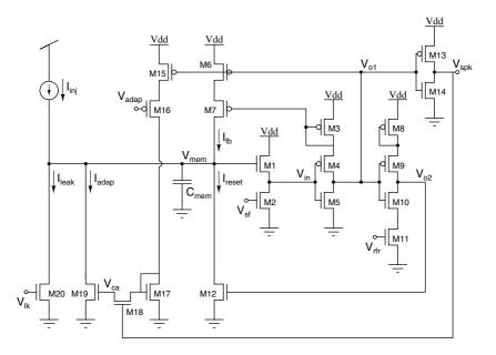
Fig. 1. Circuit diagram of the I&F neuron.
