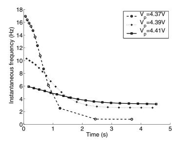
Fig. 6. Instantaneous frequency response of the circuit with  $V_{adap}$ =4.19V, for increasing values of input step amplitudes (decreasing values of  $V_p$ ). The abscissa of each data point corresponds to the spike time from the input step onset.
