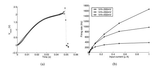
**Fig. 2.** (a) Measured data (circles) representing an action potential generated for a constant input current  $I_{inj}$  with spike-frequency adaptation and refractory period mechanisms activated. The data is fitted with the analytical model of eq. (5) (solid line). (b) Circuit's f-I curves (firing rate versus input current  $I_{inj}$ ) for different refractory period settings.
