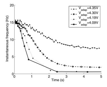
Fig. 7. Instantaneous frequency response for different adaptation rates. The neuron adapts more quickly as the adaptation rate increases ( $V_{adap}$  decreases), and the corresponding steady-state output frequency is lower.
