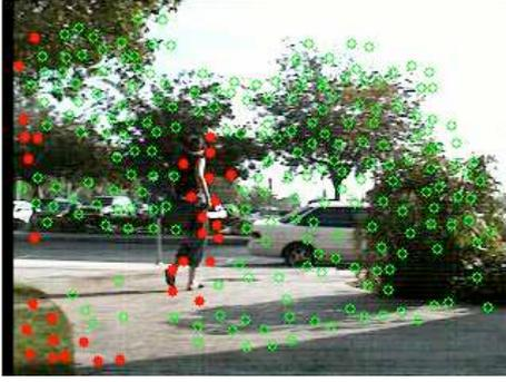
**Figure 4.4:** *Motion subsets.* The features are divided in two subsets. The one set belongs to self-moving objects (filled red circles) and the other to the background (green empty circles). (Image found in [111])
