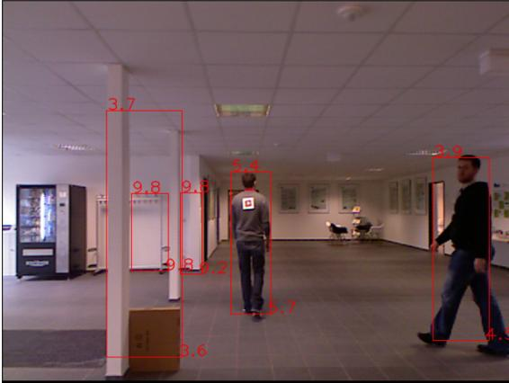
**Figure 4.17:** *u-v-disparity human detection.* The pre-detection searches for objects with similar size dimension compared to a typical upright standing human. The size is calculated through the u-v-disparity. All found objects are marked with a red rectangle. In the upper left and lower right, the minimum and maximum depth of an object is denoted. Areas with similar dimensions are also found by the pre-detection.
