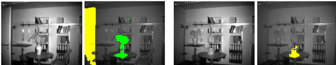
**Figure 3.10:** Two examples showing the segmented movable objects in a 2D image. The first and the third image are the original images and the second and fourth show the marked object. The coloured areas belong to different recognized objects, which have been moved at least one time.
