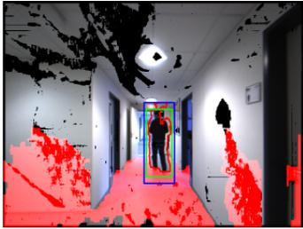
**Figure 4.1:** *Detection and Tracking of a human.* The scene is simplified through a floor elimination (in red). Afterwards, the human is detected and tracked (green and blue rectangle). In red the person is segmented from the background. The information about humans present in the scene and their movements is an essential knowledge for mobile robots in order to interact safely with their environment.
