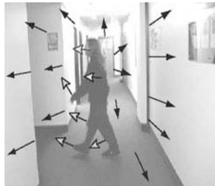
**Figure 4.3:** *Motion on a moving platform.* Motion different from the learned ego motion flow field (white arrows) indicates other moving objects. (Image found in [160])
