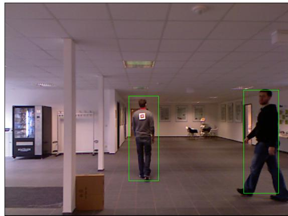
**Figure 4.19:** *Detection verification.* All hypotheses from the pre-detection (see Fig. (4.17)) are verified through the Histograms of oriented Gradients classifier. All verified detections are marked with a green rectangle.
