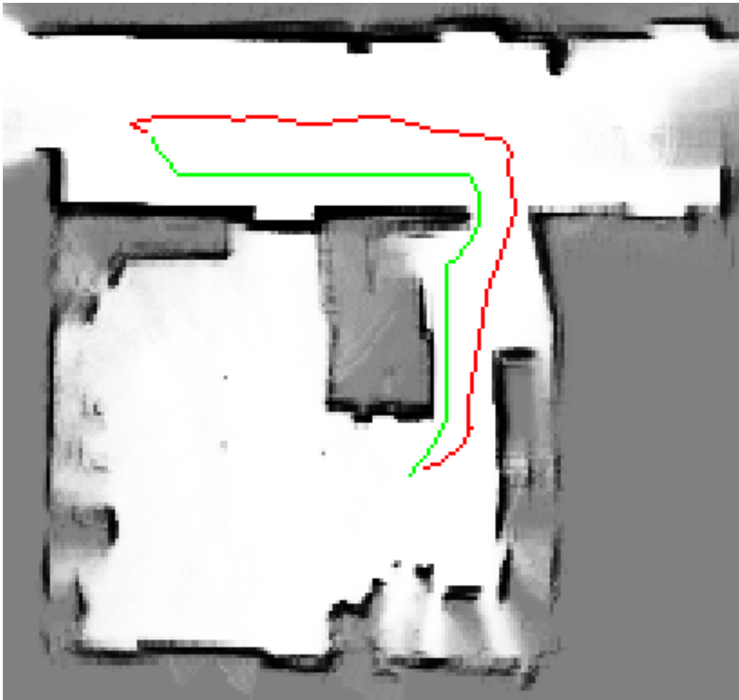
Figure 4.10.: Comparison of the path computed from NF1 and our approach for the robot from A to B given in Fig. 4.7. The green path from NF1 is close to obstacles, while the red path reveals navigation strategies of the guide-person.
