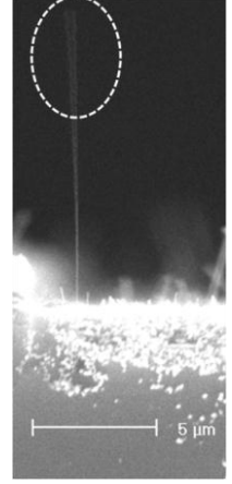
Figure 58: SEM image of an oscillating Zn NW, agitated by the imaging electron beam.
