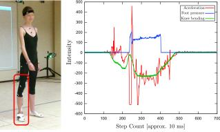
(a) Dancer equipped (b) Plot of a data sample recorded during a single with a BRIX stack. jump.
