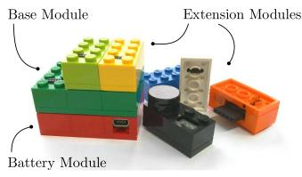
Figure 1: A BRIX stack example and extension modules.
