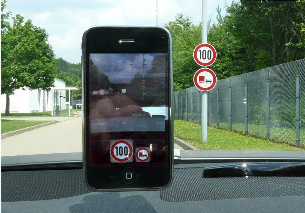
Figure A.8: Prototypical interface of traffic sign recognition ported to iPhone 3G
