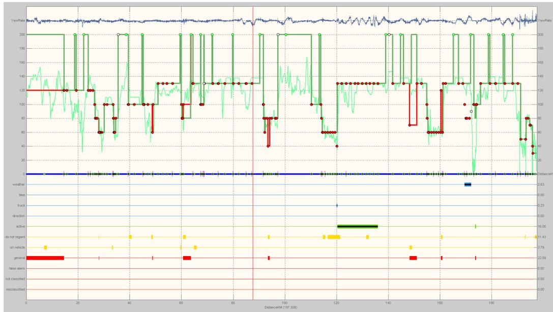
Figure 5.4: Example of a labelled route of about 200 km length with labelled auxiliary information yaw rate (top blue), travelled speed (light green), allowed speed or *ground truth* (dark green), and error of speed limit system (red)
