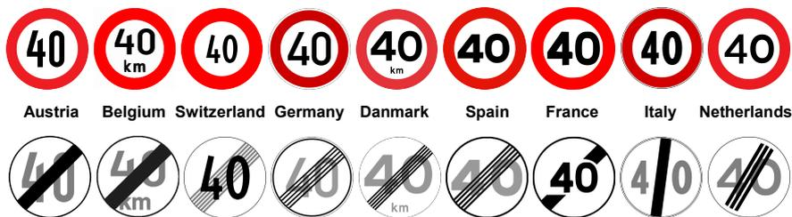
Figure 1.7: Representations of Speed Limit/End 40 km/h signs in Europe
