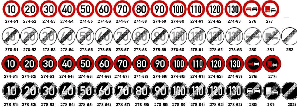
Figure A.3: Sign types and names taken from the German advice book for the placement of traffic signalisation [Bald and Giesa, 2002]
