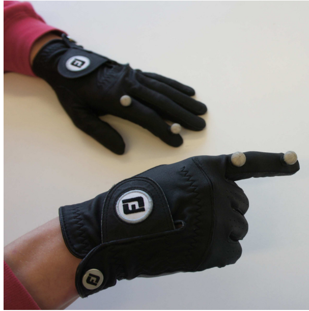
Fig. 2. Customized gloves for tracking the index fingers.
