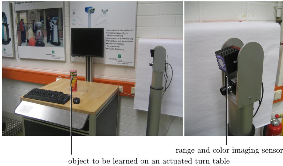
Figure 5.3: Object learning cell used in the experiments.
