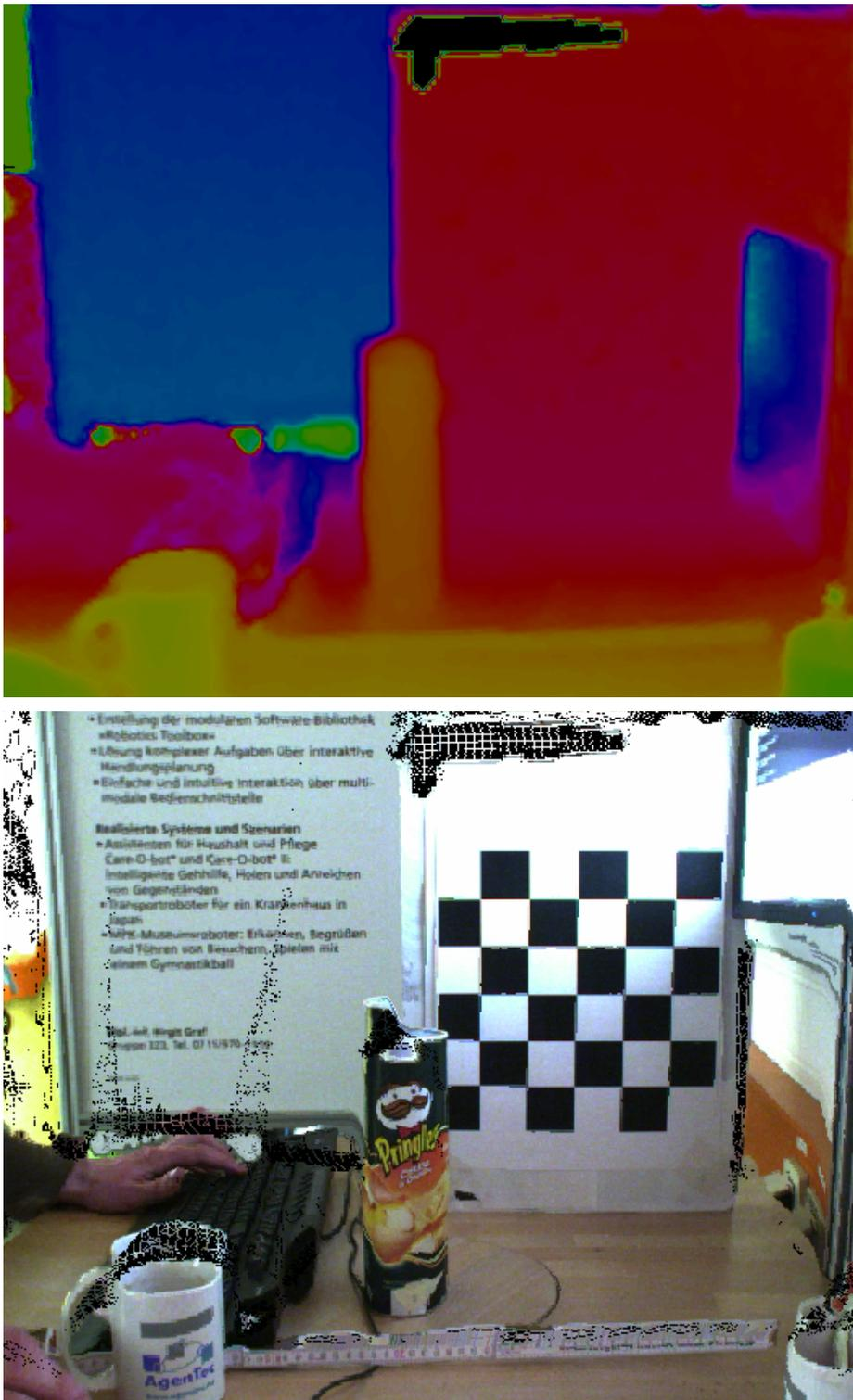
Figure 4.3: Some results of the shared image computation as suggested in this document. Top: the z-channel coded in spectral color. Bottom: the color part of the shared image (doubled areas are marked black).
