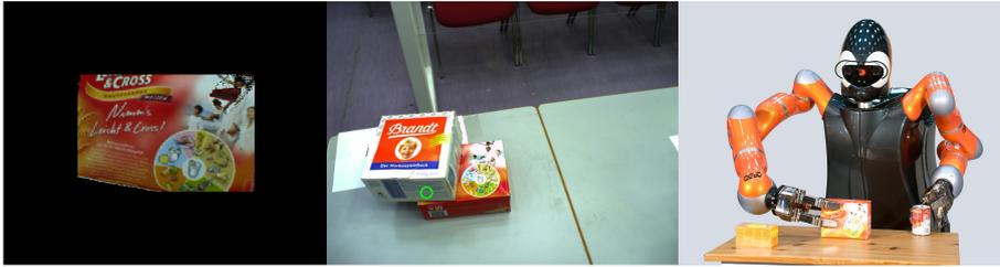
Figure 7.19: Live tests on the robot. Left: a segmented training image. Center: the object is detected even in the case of another object located on top of it. The green circle annotates the position of the detected frame. Right: the robot platform used in the live tests.
