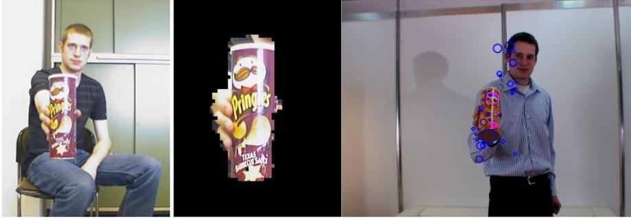
Figure 5.2: Object appearance segmentation based on demonstration. In both cases the segmentation mask is defined by a threshold in  $z$ . Left: the pixel values are masked. Right: masking is done on feature point level; purple rings annotate accepted feature points and blue rings rejected ones.
