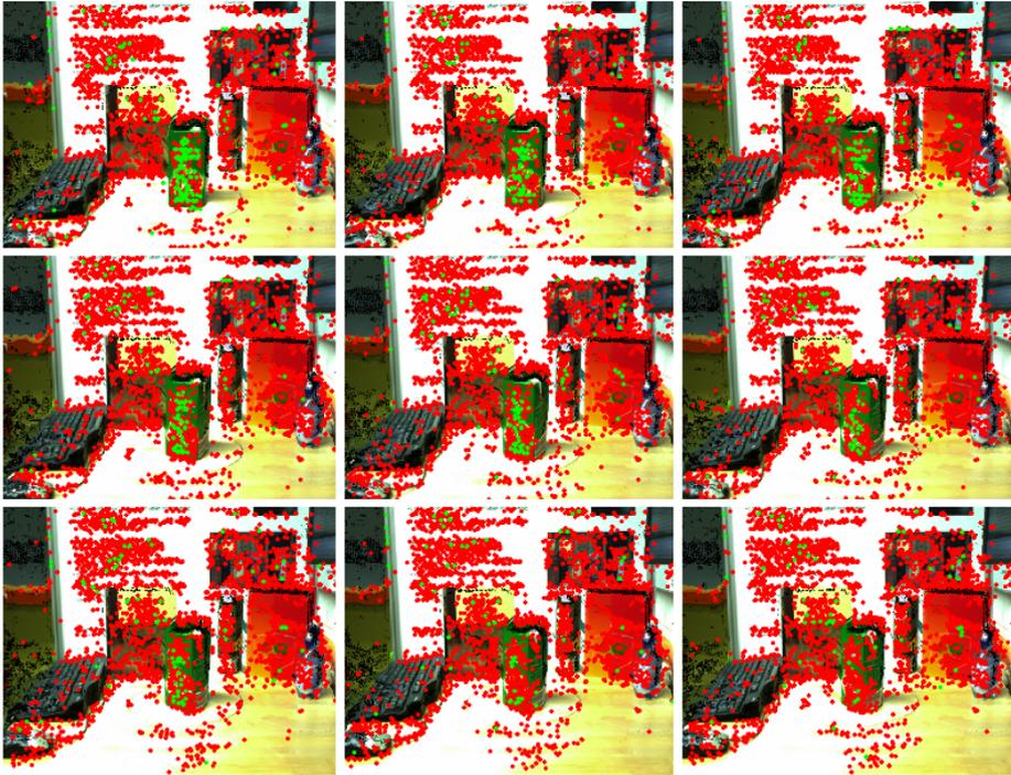
Figure 7.10: A visualization of the SURF descriptor stability. The first 9 images of the object database (object: juice,  $5^\circ$  rotation) are shown. Only the descriptors of the first image are taught and then matched with the subsequent images. Stable descriptors (green points) exist up to about  $40^\circ$  rotation
