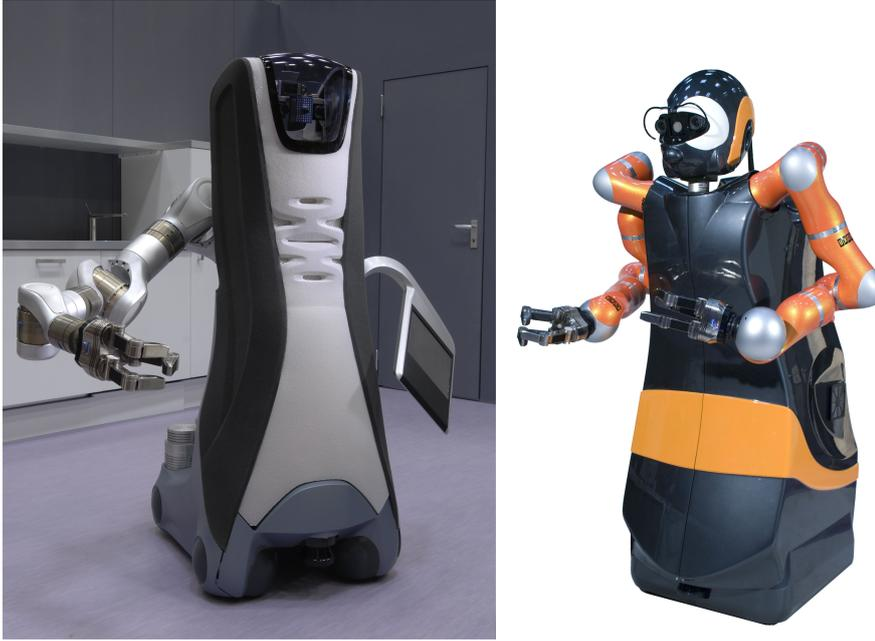
Figure 1.1: Two examples of service robot research platforms. On the left the Care-O-bot<sup>®</sup> 3 is shown and on the right a newer platform that includes two manipulator arms. Both robots are equipped with various sensors and actuators and were used during the work related to this document.
