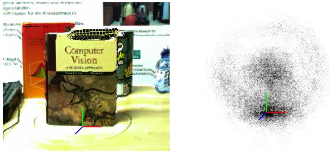
Figure 6.4: This figure shows the set of hypotheses  $H$  for an object model of a book. Left: the scene (color part of the shared image) containing the book. Right: the dots represent the  $x$ - and  $y$ -coordinates of the base point of each frame hypothesis. The red, green, and blue lines in the left and right image represent the object reference frame (left image) and the result frame (right) that are manually annotated in this figure.
