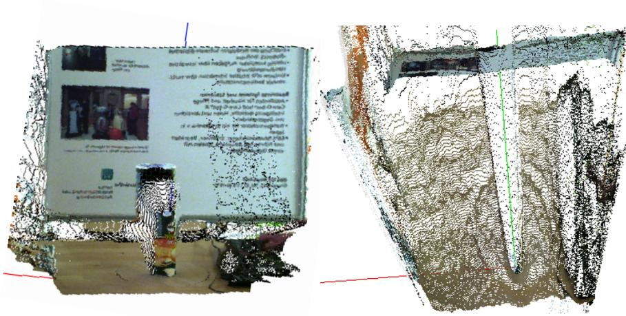
Figure 4.4: 3D views of a Shared Image. Left: front view of a scene containing the cylindrical crisps box. Right: the same scene from a bird's perspective. The red, green, and blue lines in the background are the  $(x, y, \text{ and } z)$  axes of the reference coordinate system.
