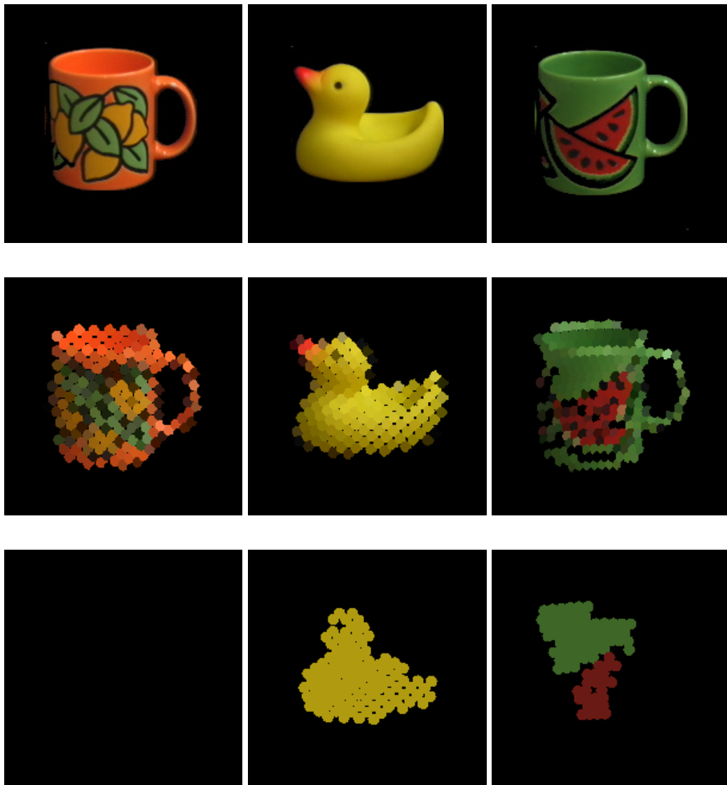
Figure 5.5: Regions of objects. The examples come from Fig. 5.4. Top row: object images. Middle row: feature map representations. Bottom row: resulting regions. Left column: As the feature map representation shows, the cup is too inhomogeneously structured in color, so the model is not able to find a large enough homogeneous color region. A more foveal representation of the cup could lead to a different result, as it would be mapped by more pixels (see Fig. 5.7). Middle column: Almost the whole duck is represented by one single region. Only the beak gets lost. Right column: The cup is represented by two regions, as it consists of two large enough homogeneous color regions.
