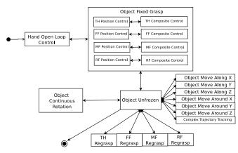
Fig. 5: Human Robot Hand Interaction Object Manipulation statechart
