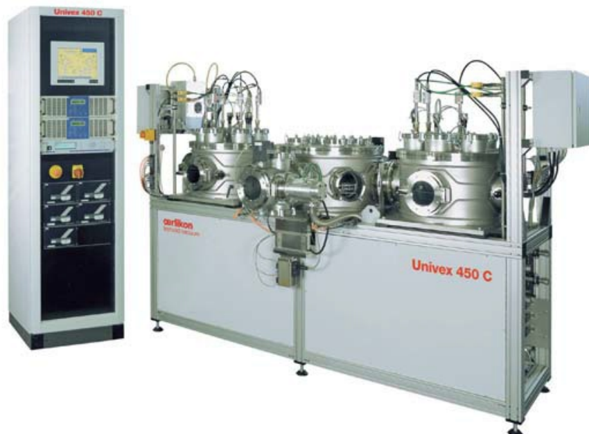
Figure 20: Leyboldt UNIVEX cluster sputter machine with two deposition chambers.
