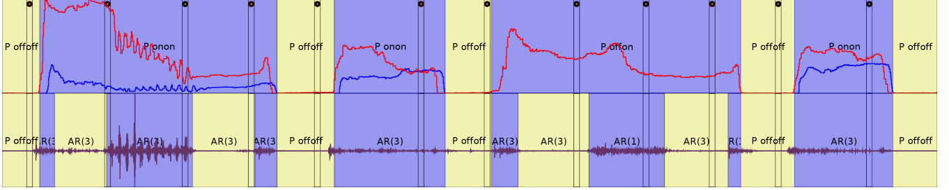
Figure 2: Initial segmentation and "subordinate" sub-segmentation for one multimodal time series. The first row shows the result of applying Fearnhead’s method with joint threshold models of the tactile data of both hands (see Sec. 3.2.1 for details). The segmentation is overlaid with the tactile signals of both hands. The second row shows the refinement of the segmentation in the first row that is computed by applying Fearnhead’s method to the audio signal within each "contact" segment (see Sec. 3.2.2 for details). In the second row the segmentation is overlaid with the audio signal.
