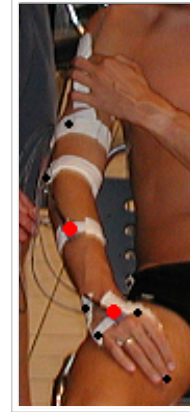
Figure 2: Sensor setup used to measure the pressure data at hand palm, hand back, elbow and shoulder.
