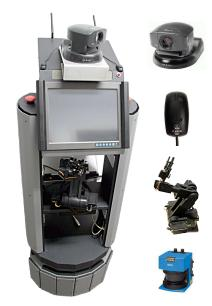
Fig. 1. The robot ToBI with it's components shown on the right. From top right: Pan-/Tilt-camera, interfacial microphone, Pioneer 5DOF arm and laser range finder.
