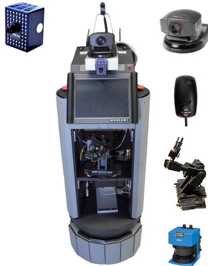
**Fig. 1.** The robot ToBI with its components shown on the right. From top right: Pan-/Tilt-camera, interfacial microphone, Pioneer 5DOF arm and laser range finder.
