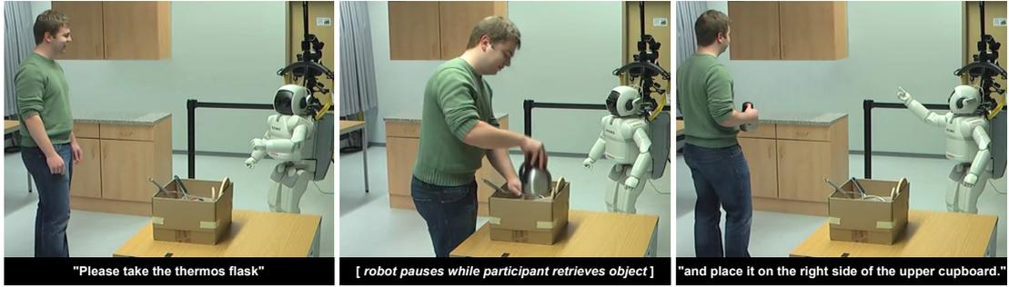
**Figure 8.1:** Modified experimental design with split utterances: the robot’s utterance delivery is paused after the first chunk until the participant has retrieved the object.
