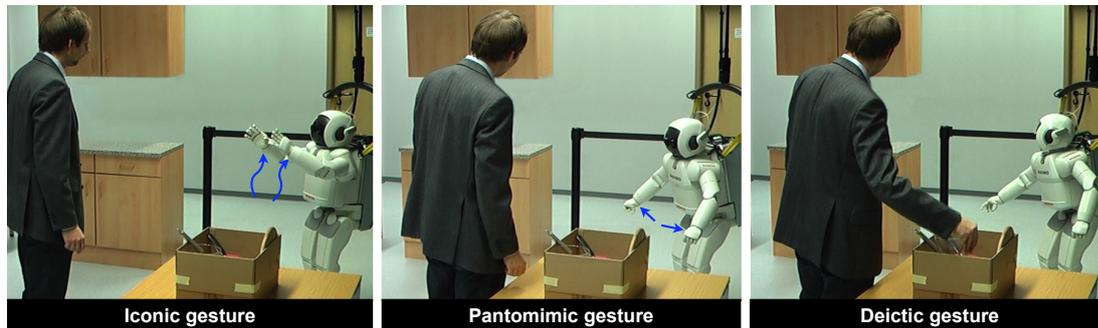
**Figure 7.3:** Examples of the three types of gesture performed by the robot during interaction in the multimodal conditions (left to right; blue arrows indicating the movement trajectory and direction of dynamic gestures): *iconic gesture* illustrating the shape of the vase; *pantomimic gesture* conveying the act of opening the lower cupboard; *deictic gesture* pointing at the designated location (adapted from Salem et al., 2011c).
