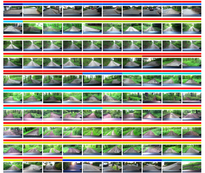
Figure 5. Assignment of episodes. The video is represented by 100 test images taken at every 600th time step (left to right and top to bottom). The colour bars over each image visualise the assignment of episodes for two different networks (top bar: \rho_a=0.5 ; bottom bar: \rho_a=0.7 ; remaining parameters for both networks: \beta_{sbm}=0.25 , \phi=5 , \tau=200 , t^{max}=400 ). Each episode is denoted by an individual colour.
