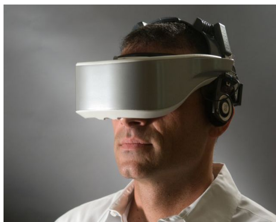
Figure 2.1.: Sensics zSight HMD 1 . The zSight provides 70 degree field of view, an integrated head tracker, audio and microphone.
