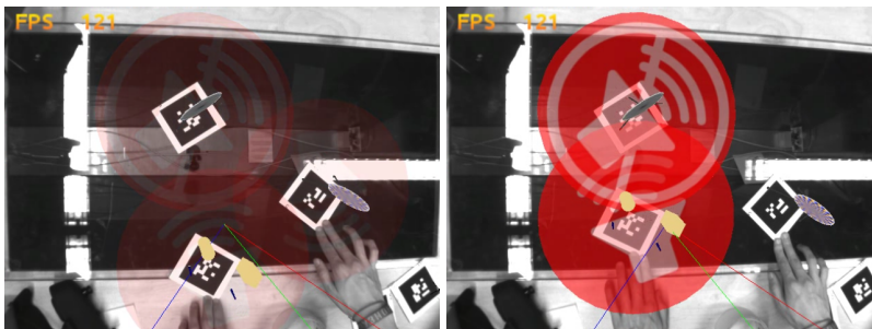
Figure 5.10.: Constraint evaluation. Two stages of constraint violations are shown from top view. The left picture shows minor constraints violations caused by multiple objects. On the right picture more severe constraints violations resulting in less transparency of radius disks are shown.
