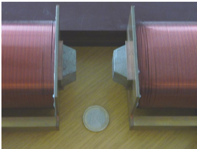
Fig. 3.3: Image of the coil setup for magnetic field generation
