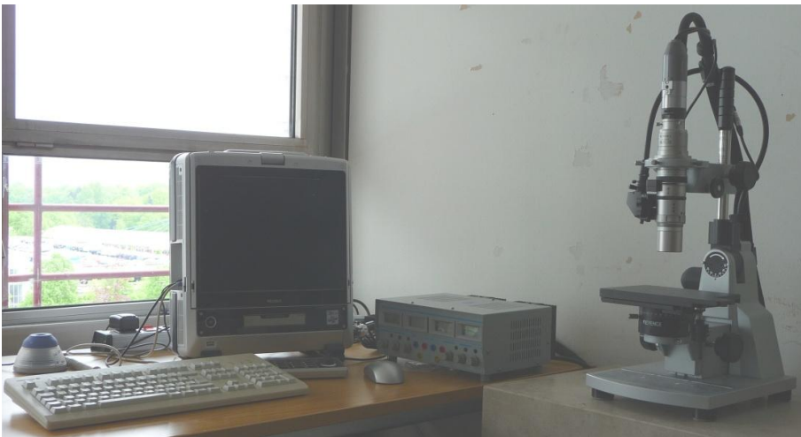
Fig. 3.2: Optical microscope Keyence VHX-600 with VH-Z100UR zoom objective.
