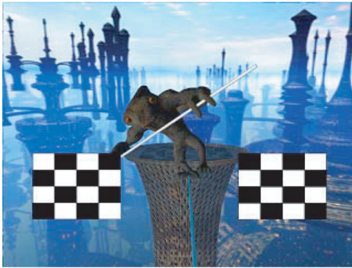
Figure 2.10. Pole balancing task controlled by SSVEP. The stimuli for left and right movements are phase inverted checkerboard patterns, flickering at a specific rate.
