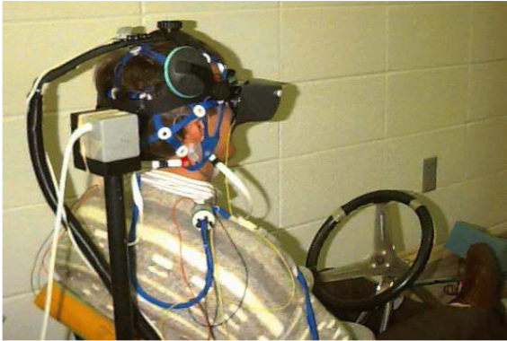
Figure 3.9. The virtual stoplight experiment by Bayliss. Subjects were sat in a modified go-cart (left) and were required to attend to red light to stop driving in a virtual street (right).
