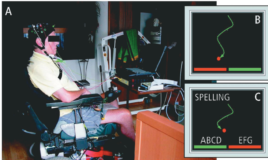
Figure 3.4. A BCI based on slow cortical potentials operated by a patient suffering from amyotrophic lateral sclerosis .
