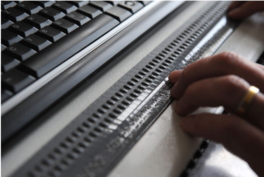
Figure 1.1. Braille-Displays allow visual impaired people to read the content of a computer screen by using tactile-coded alphabets.
