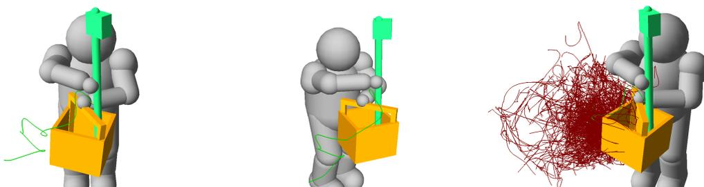
**Figure 7.13:** Example of a solution path to target position 3. The flower trajectory is shown in green and the search tree in red.
