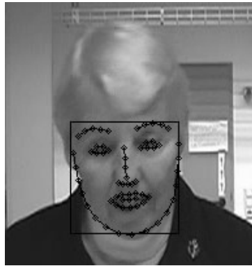
Figure 4.5.: Example of a constrained local model fitted to a target image. Please refer to Sec. 4.5.2.
