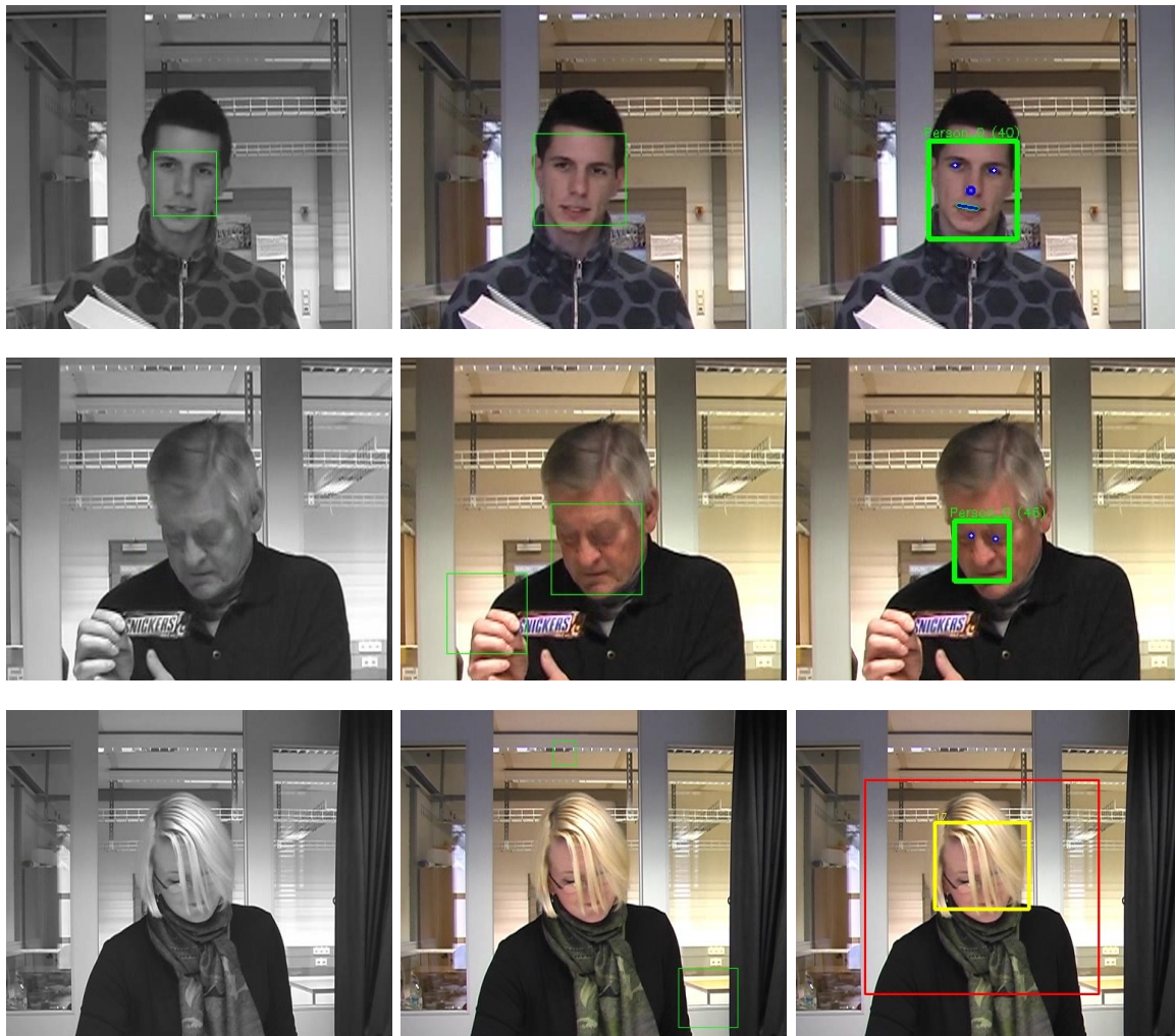
Figure 5.1.: Typical face detection results for object-teaching videos of the boost detector of Peters [400] (left), OpenCV 's boost detector [40] (middle), and the Encara detector [64] (right). Top row: an easy case where all three detectors find the face and Encara additionally locates eyes, mouth, and nose. Middle row: a more difficult case with a rotated face which is slightly out of the training range of Peters' boost detector, whereas the OpenCV detector finds the face but also an additional false positive, and the Encara detector locates a little too small bounding box without nose and mouth and rough eye positions only. Bottom row: a hard case where the head and shoulder detector of the Encara approach is able to detect the face roughly nevertheless, while the others cannot find it due to the occlusion caused by the hair. Please refer to Sec. 5.1.
