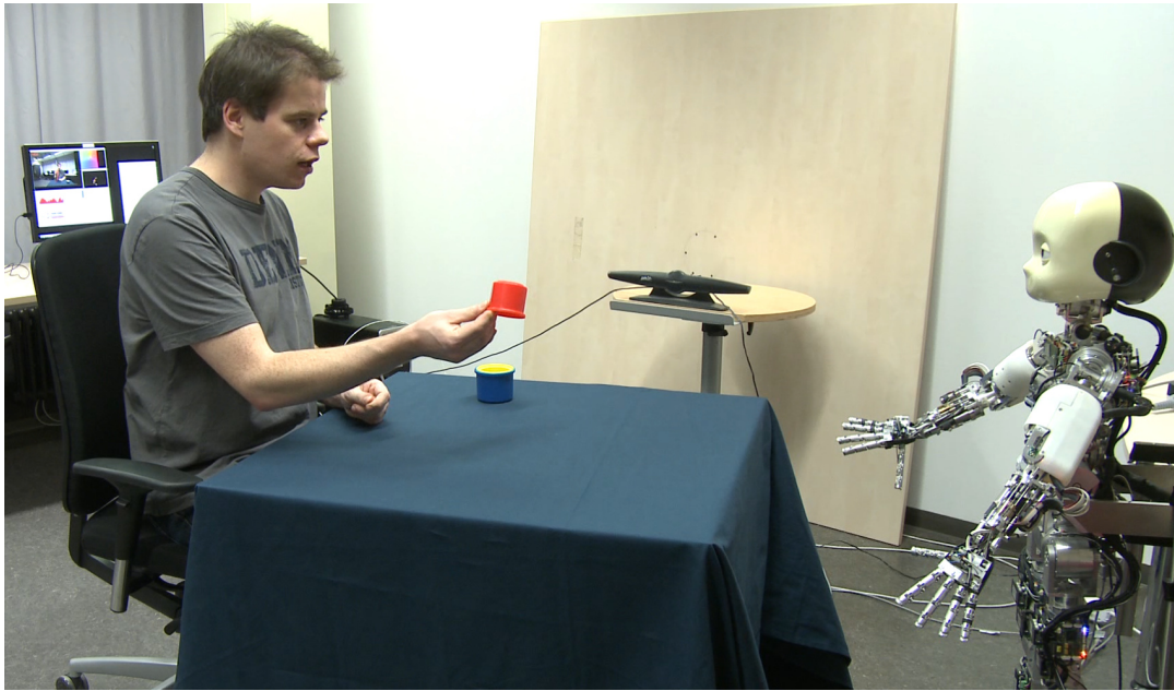
Figure 6.6.: A human user demonstrates cup stacking to the iCub robot. The iCub observes the scene through one of its eye cameras. Speech is recorded using an external microphone (middle). Visualization tools of the acoustic packaging systems are displayed on the screen in the background.
