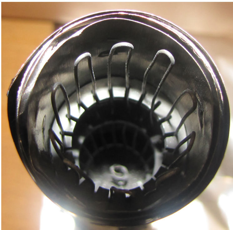
Figure 55: Topview into the heating part of the Knudsen cell which encloses the crucible.
