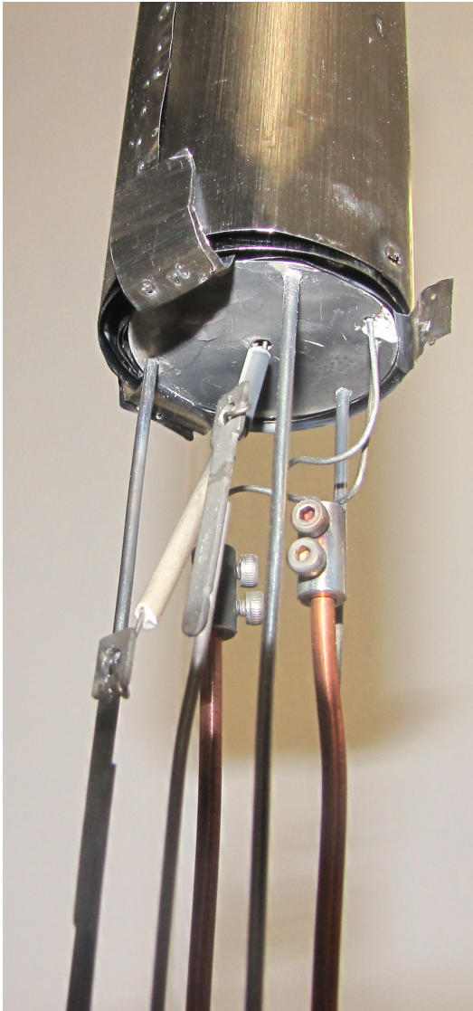
Figure 54: Detailed view onto the lower side of the holding pan with heating wire connections and thermocouple wires welded to the feedthrough contacts.
