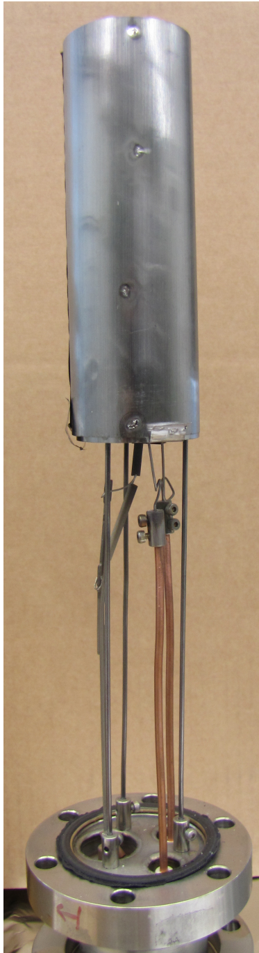
Figure 53: Side view of an older, slightly different version of the custom made Knudsen cell. The mounting of the thermal shielding is not completely screwed but is held in place by Ta flaps screwed to the holding "pan". Furthermore the threaded rods of the final version are stronger.
