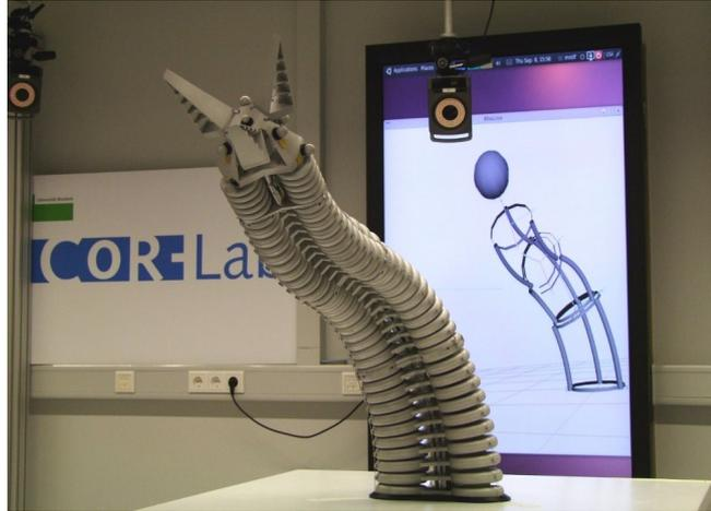
Figure 1.1: The *Bionic Handling Assistant* mimics an elephant trunk.
