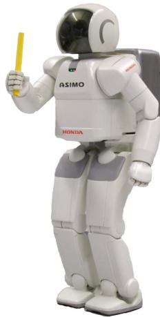
Figure 5.8: Humanoid robot morphology used for reaching in 3D. *Figure from [Rolf et al., 2010b].*
