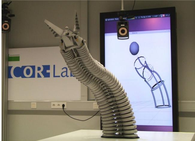
Figure 7.1: The *Bionic Handling Assistant* mimics an elephant trunk.
