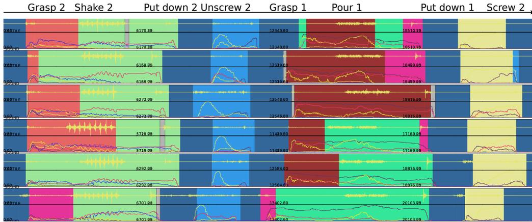
Figure 6.8: An example of label assignment for clustering with a combination of tactile and joint-angles modalities. Labels are designated by random colors.
