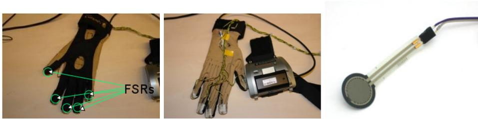
Figure 3.1: Proprioceptive hand sensors. Left: Immersion CyberGlove II with FSR sensors attached to the fingertips. FSR sensors are covered with a layer of foam to achieve a better distribution of force. Middle: Immersion CyberGlove II from the back. The cables connecting the FSR sensors with the Bluetooth communication module are mounted on the back of the hand to avoid movement restrictions during object manipulation. Right: FSR-402 sensor used on each fingertip for capturing of pressure.
