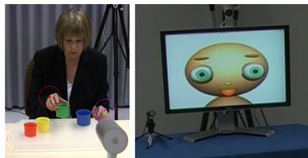
Figure 3.7: In the left picture, the red and violet circles depict the tracking regions which are tracked by the hand tracker system. The points in the middle of the circles are the resulting points for the 2D hand trajectory. In the right picture, the virtual robot used is shown.
