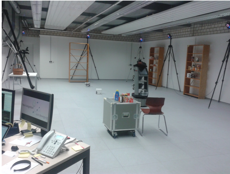
Figure 8.1: The picture presents the dimensions of the crossing area and the setup of the shelves. The shelves and the storing place were set up in a way that the confederate, who played a customer and the robot would coincidentally cross each other's way in 45° and 90° angles. The picture displays the VICON cameras on tripods. Boxes in the middle of the area present the obstacles for the practise of the participants before they started a trial. These are removed for the actual trial.
