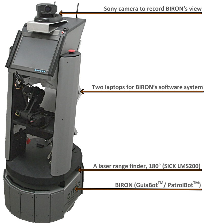
Figure 5.3: This figure depicts the robot BIRON - the (BIlefeld Robot companiON). The robot is a combination of a two-wheeled PatrolBot™ and GuiaBot™ by Adept MobileRobots. The on-board camera is used to record BIRON's view for later video annotation. There is a laser range finder (SICK LMS200) inside the base front with a scanning range of 180° and scanning height at 30 cm above the floor. The arm with gripper was not used and folded up during the study.
