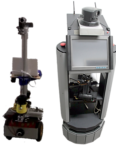
Figure 1.3: The mechanical-looking robots Snoopy (left) and BIRON (right) are used within the studies examining the communicative aspect of motion in HRI. Section 5.1.4 provides more information on BIRON and Section 6.1.3 more on Snoopy. These robots are able to rotate their body and move forwards and backwards. Subtle motions of these robots can communicate their intent, see Chapter 3.
