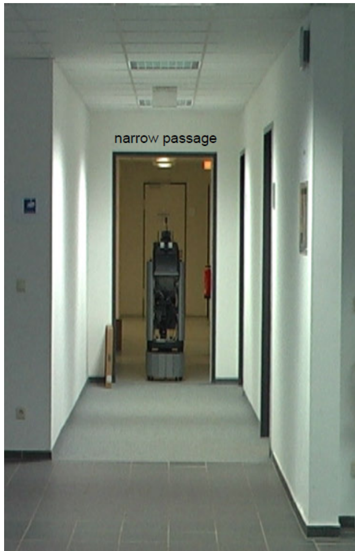
Figure 5.2: This figure displays the robot BIRON in the corridor at the narrow passage (fire door frame). This corridor is 1.85 m wide and about 12.63 m long. The fire door frame creates a spatial bottleneck of 1.15 m. This leaves approximately 32.5 cm on each side of BIRON standing in the middle of the door frame. During the trials, participants turned into the corridor from the right bottom edge of the picture. This picture also presents the initial view of the participant when he / she turned into the corridor. The picture also presents the view of the external camera during the trials. In addition, it depicts the robot BIRON in its initial position within the static setting cf. further descriptions, in particular, Section 5.1.5.
