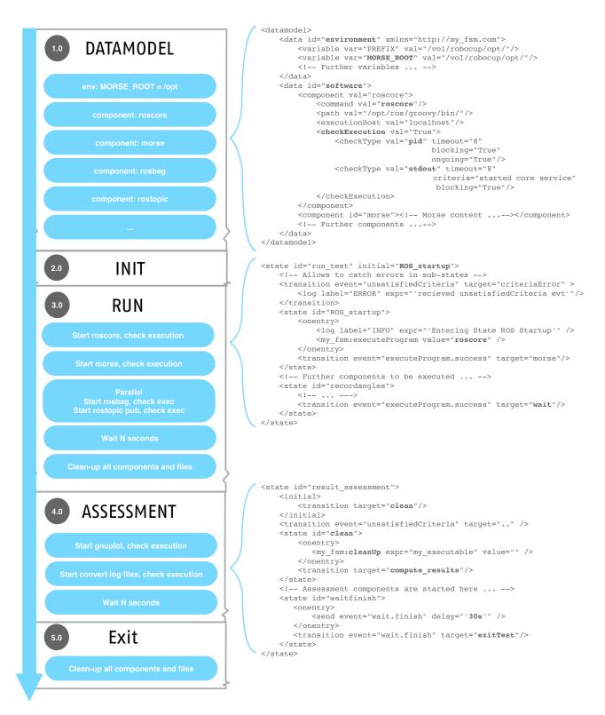
Fig. 1: Schematic state-machine based system test.
