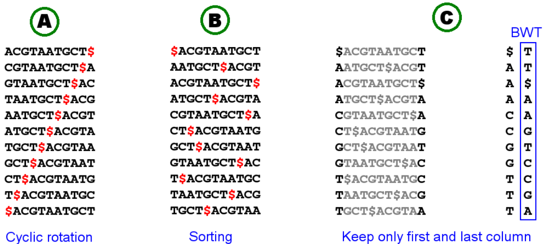
Figure 5.3.: Naive approach to create a Burrows-Wheeler transformation (BWT) of a text, in this case the DNA sequence G : “ACGTAATGCT”. (A) First a special character \$ is appended to the sequence, and a matrix of all cyclic rotations is created. (B) The matrix rows are sorted lexicographically. (C) All columns except the first and the last one are discarded. The last column is the BWT, the first column is needed for basic operation like the decoding of the BWT.
